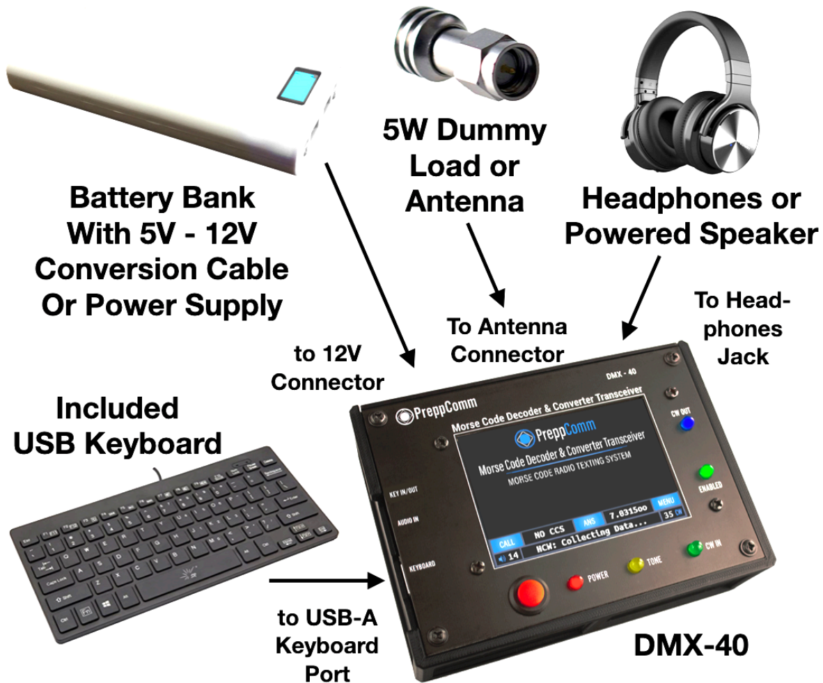
FIGURE 1: STATION SETUP AS STAND-ALONE STATION
